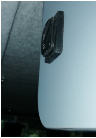
Above: Side door LED double pole switch
