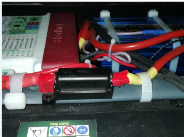
Above: Main Fuse for the Leisure Battery feed to the Isolator Switch (60A)
